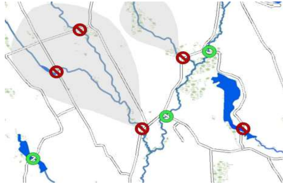
Upstream culverts providing flood storage and moderating peak flows?
