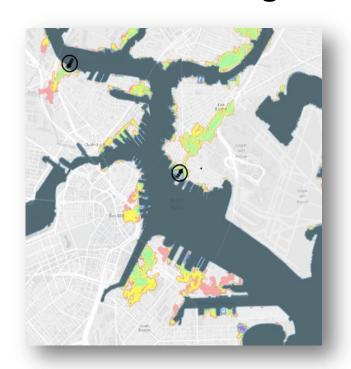
Figure 6-1. Flood entry point locations that are viable sites for regional adaptations under the 2013 scenario (Milton site not shown).
