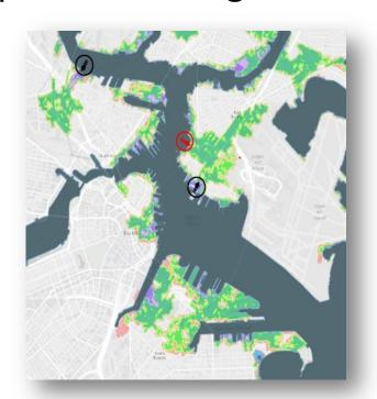
Figure 6-2. Flood entry point locations that are viable sites for regional adaptations under the 2030 scenario.
